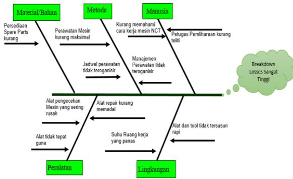
Gambar 7. Fish bone diagram breakdown losses
