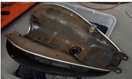
c. Final state after application of corrosion inhibitor
