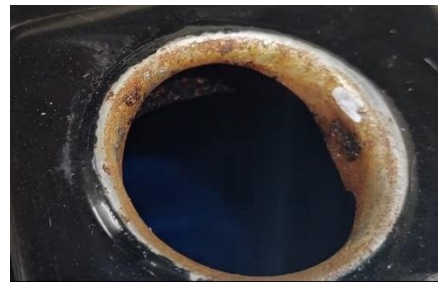
Figure 5. Intermediate rust dissolution stage after 24 hours of acid exposure.
