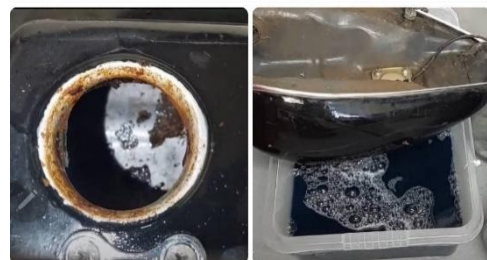
Figure 8. The tank's interior after 24 hours of exposure to the acid cleaner. Partial rust removal is evident, with suspended particles visible in the solution
