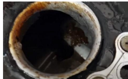
Figure 5. Intermediate rust dissolution stage after 24 hours of acid exposure.
