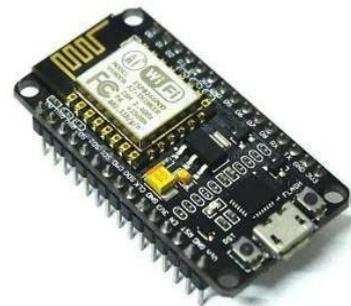
**Gambar 3.** NodeMCU ESP8266 ESP-12E
