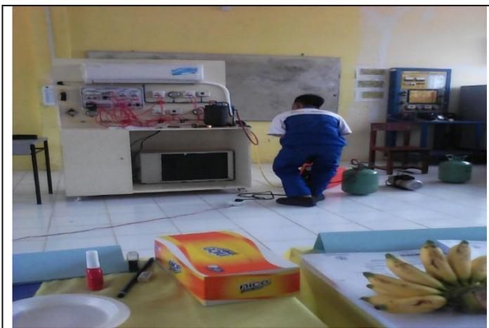
Gambar 4.21 Test Kerja Trainer Simulator Air Conditional R22
