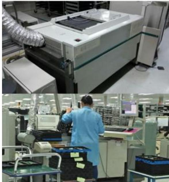
Gambar 1 proses *testing* ICT
