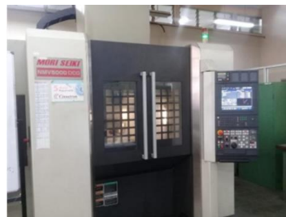
Gambar 1. Mesin CNC milling mori seiki nmv 5000 dcg
